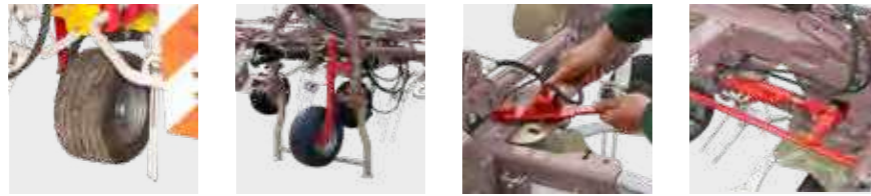
Tyres 16 x 9.50-8 inner rotor Jockey wheel T 16" Mechanical fenceline system Hydraulic fenceline system
